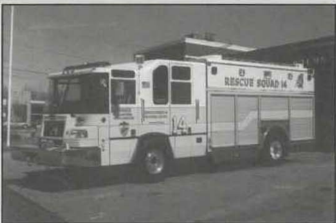
In January of 1997, Burke's 1991 Duplex/Saulsbury heavy squad caught fire while sitting in the apparatus bay, significantly damaging other apparatus and doing extensive damage to the Burke fire station. Pierce rebuilt the truck with a new 1998 Quantum chassis. The Saulsbury box was rebuilt by Pierce and had roll up doors installed. (Mike Sanders photo).
