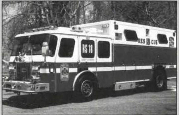
In 1984 and 1986, Fairfax County purchased squads built on Ford C chassis. The 1984 truck was sent back to Emergency One in 1995 and received a brand new Emergency One Protector cab and was placed in service as Rescue Squad 18. The 1986 squad had a similar conversion and is in service at Station 26. (Mike Sanders photo).
