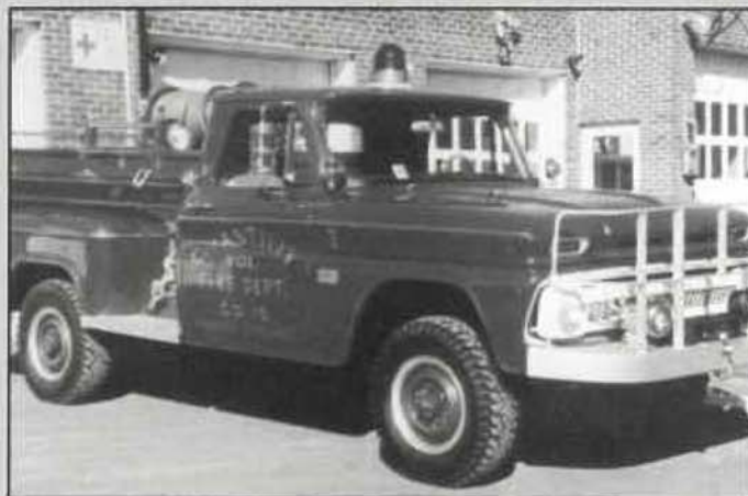
Chantilly's brush truck was once a 1966 Chevrolet pick up complete with a 300 gpm pump and 150 gallons of water. (Mike Sanders photo).
