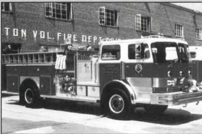
Lorton purchased the first top mount pump panel engine in the Northern Virginia area. Wagon 19 was a 1982 PemFab/Emergency One with a 1250 gpm pump and 500 gallons of water. Wagon 19 was rehabed in 1993 by Emergency One and returned with a new Hurricane chassis. (Mike Sanders photo).
