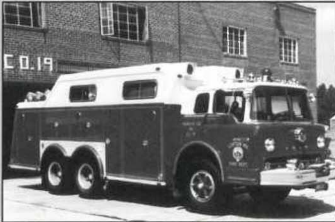
Lorton's heavy squad once ran this 1973 Ford C/Swab (400 gpm/300 gwt) until 1988 when a new Emergency One squad replaced it. The Ford was sold to a department in Pennsylvania. (Mike Sanders photo).
