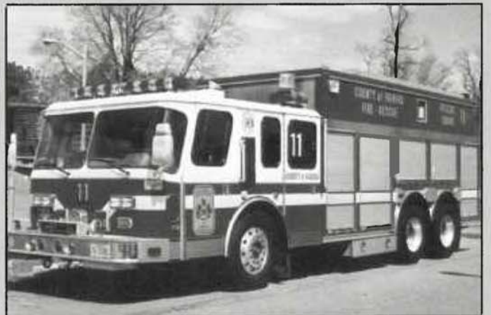
Rescue Squad 11 received a 1990 Emergency One Hurricane with roll up compartment doors and tandem rear axle. (Mike Sanders photo).
