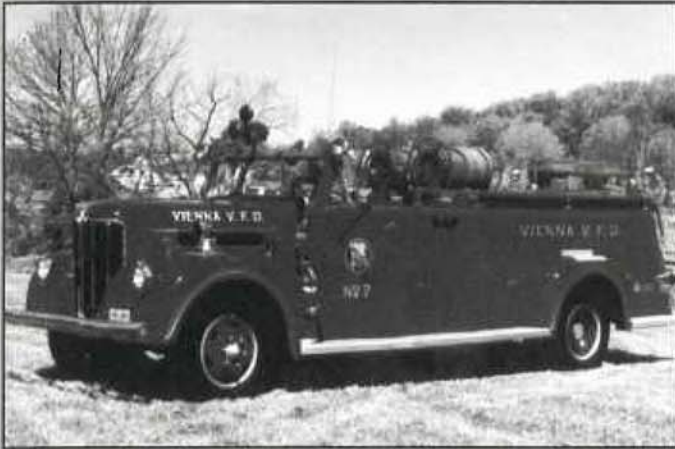
In 1946, Vienna purchased this 500 gpm Maxim pumper. It was later sold to another department in Virginia and purchased back by Vienna to be fully restored during 1997. (Mike Sanders photo).
