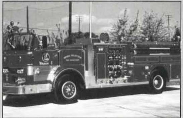
Vienna's 1970 Duplex/Young 1000 gpm pumper eventually had a roof added to it in the early 1980s. (Mike Sanders photo).
