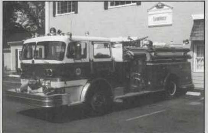
In 1973, Fairfax County purchased 5 Imperial pumpers (1000 gpm/500 gwt). During 1982 and 1983, Emergency One rebuilt all of the trucks. (Mike Sanders photo).
