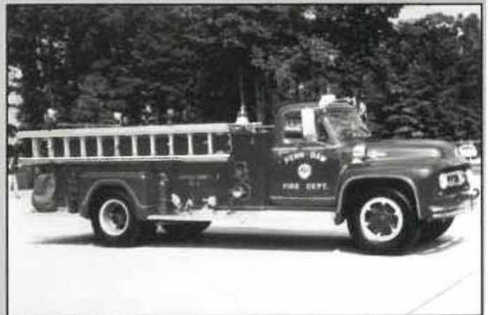
Penn Daw's 1953 Ford/Oren 750 gpm pumper was later converted into a light unit, Vienna, which owned a 1956 Ford, also had a similar conversion done on their pumper. (Mike Sanders photo).
