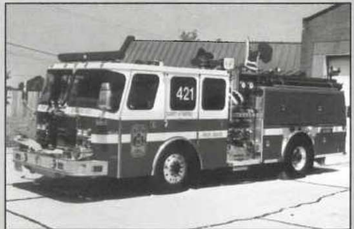
Engine 421 is a representation of the current type of county purchased engines. This 1998 Emergency One Cyclone model as a 1250 gpm pump and carries 750 gallons of water. (Mike Sanders photo).
