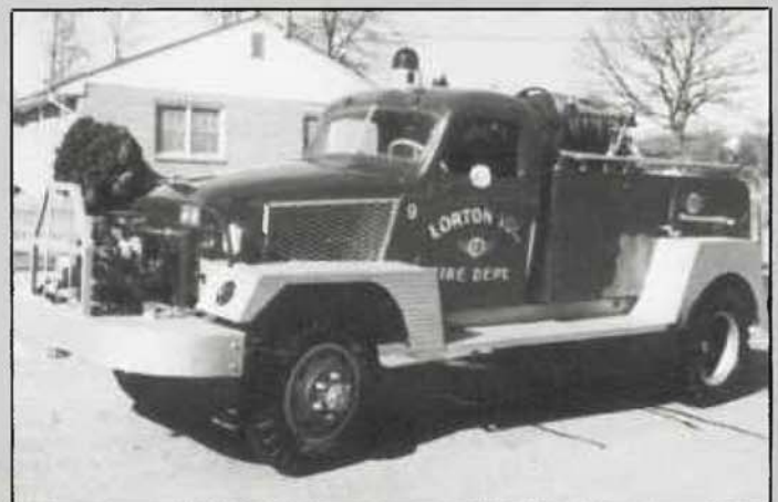
Lorton had several old military brush trucks. This 1942 Chevrolet had a front mount 300 gpm pump and carried 300 gallons of water. (Mike Sanders photo).
