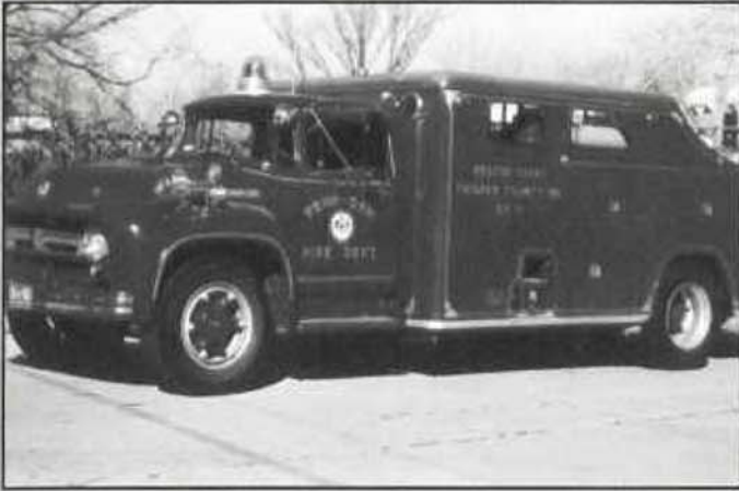
Penn Daw's unique 1956 Ford/Oren heavy rescue squad complete with a 250 gpm pump and 250 gallons of water. (John Floyd photo).
