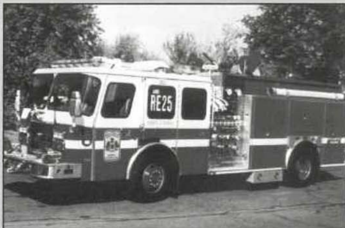
During the 1990s, the rescue engine concept (combination fire engine and rescue squad) became increasingly popular. Reston Company 25 received a 1994 Emergency One 1250 gpm rescue engine complete with a 750 gallon water tank. (Mike Sanders photo).
