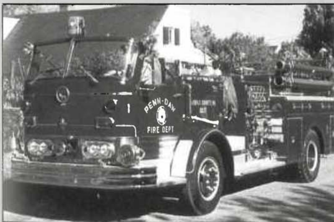
Penn Daw's beautiful open cab 1961 Mack C had a 1000 gpm pump and held 500 gallons of water. This Mack was later wrecked in 1964, rebuilt, and returned to service with an enclosed cab. (Pete West photo).
