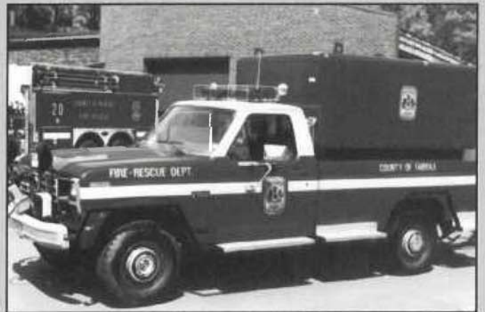
Two 1985 Ford F/Steeldraulic trucks were purchased by Fairfax County. These trucks could serve two purposes - a small ambulance body could fit in the bed or a skid mount to convert the truck into a brush fire unit. This Ford ran as Brush 20 and was also used to tow Boat 20. (Mike Sanders photo).
