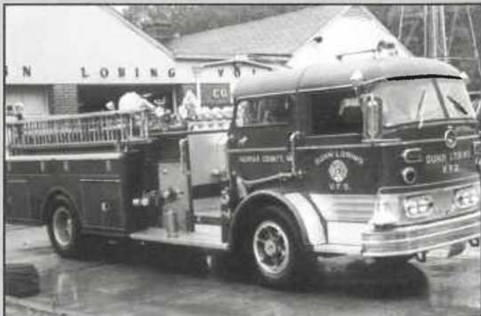
This photo was taken in 1967 in front of Dunn Loring's old fire station. It is a 1960 Mack C pumper (750 gpm/500 gwt). (Mike Sanders photo).
