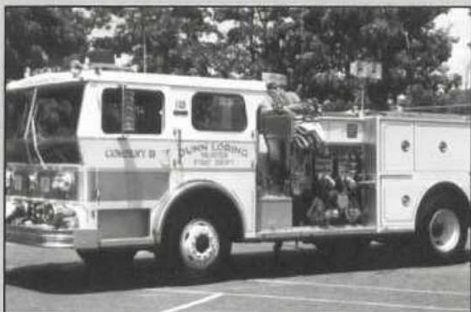
In 1976, Dunn Loring purchased two identical yellow and white Ward LaFrance 1500 gpm fire trucks. One of the Ward's was rehabed in 1983 by Pierce. (Mike Sanders photo).
