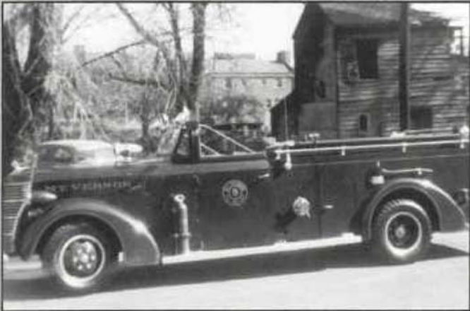
Mt. Vernon Company 9 ran this 1945 American LaFrance 500 gpm open cab pumper. (Pete West photo).
